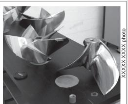
Axis machines/ Mitsubishi EDM machines are able to cut the center keyway and spline out of the 13-8 stainless steel material, to within a tolerance of .00025. They are also making props for offshore racers, turbine casings, turbine disc's and blades, and other various boat/aircraft industry related parts.
